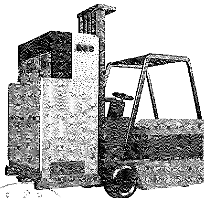
Figure 2.4: CGMCOSMOS cubicle lifting with a forklift truck
